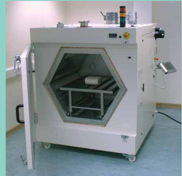
Figure 2. SEAM's 1 m 3 cavity MW furnace allows large components to be processed.
